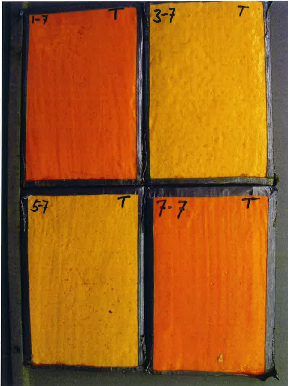
Photo 3. Panels of coating systems 1, 3, 5 and 7 after Thermal insulation and 2000 hours Salt spray test
