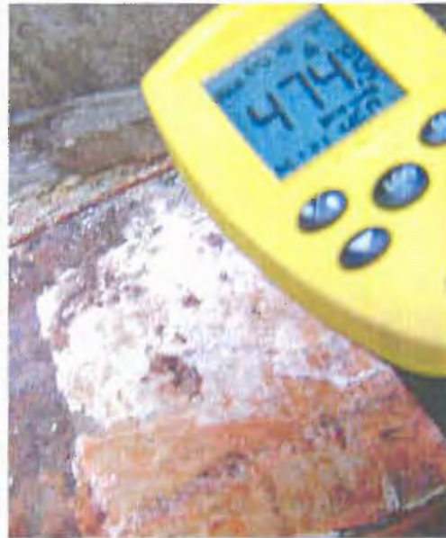
Surface temperature before HPC application: 474 C
