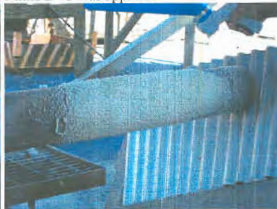
A temperature reduction from 400C on the bare pipe to 50C after the final build coat @ 250 mils DFT TOTAL was applied.
