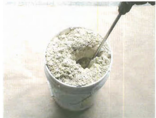
HPC – Early Stage During Mixing In Pail
