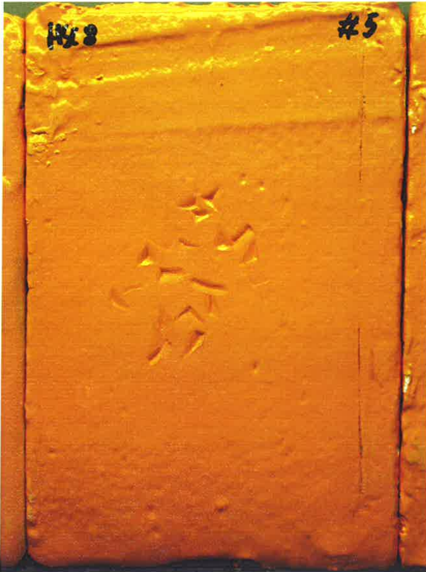
Photo 1. Panel of coating system 3a (8 mm isolation) after Impact Resistance test.
