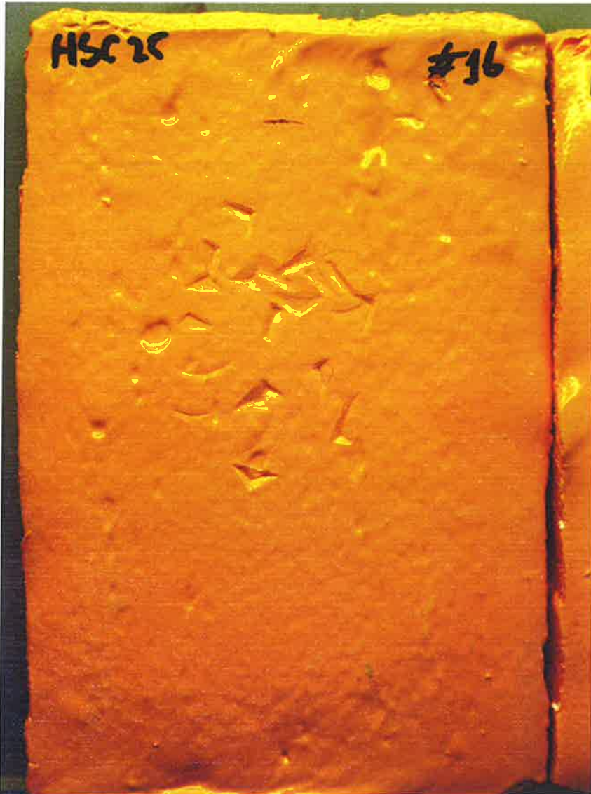
Photo 3. Panel of coating system 3c (25 mm isolation) after Impact Resistance test.
