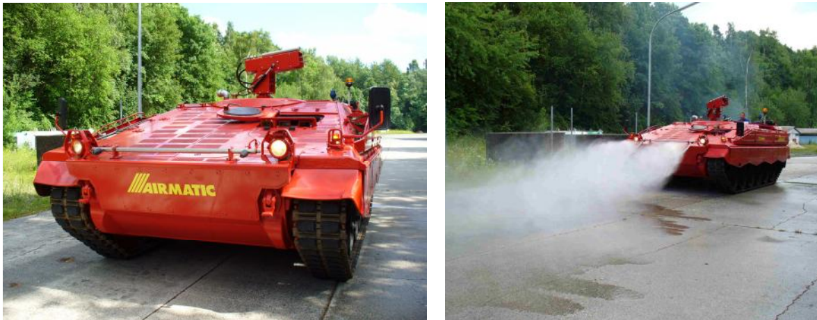
Figure 5: Basic fire-fighting vehicle on the basis of the Marder A3 armoured tank, right, and same vehicle with self-protection unit for the vehicle at the front
